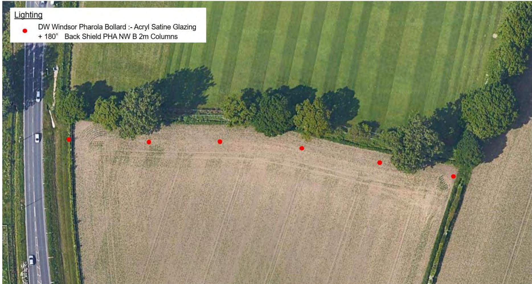
*Figure 5-5 – Visual Representation of Proposed External Lighting Model Western Field*
